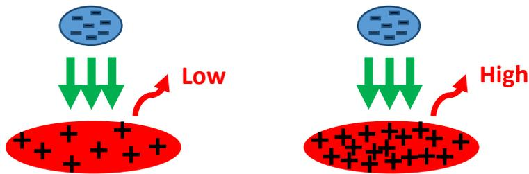
**Figure 2. Illustration of thin-target (left) and thick-target (right) bremsstrahlung.**
